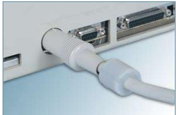
I/O cable with RFI suppressor.
