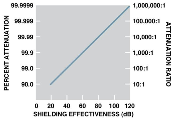
The measure of this ability to attenuate RFI is Shielding Effectiveness, SE, which is expressed in decibels, dB, the ratio of field strength on one side of the shield to the other side. The figure above shows the relationship between shielding effectiveness (in dB), the amount of attenuation, and attenuation percentage.
