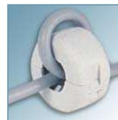
fig. 4 Increased impedance; multiple turns ( $N^2$ ) vs. one turn through ferrite; i.e., 2 turns ( $2^2$ ) = 4 times impedance
