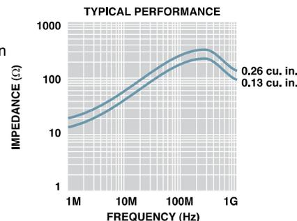
fig. 3 Two turn loop through ferrite increases effective magnetic path. Impedance increases by the square of the number of turns ( $N^2$ ).
